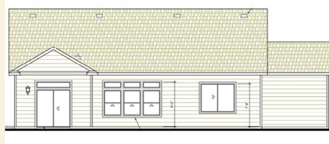
Rear Transom Windows
